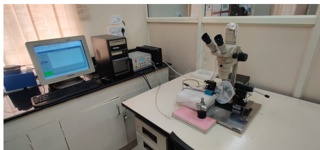
Fig. 2. Electroantennogram (EAG) system used in the experiment
