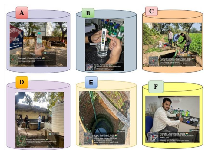
Fig. 8: A) Water Sample taken at Ramgarh Block office well; B) Konvio Kit used for TDS and EC; C) Water Sample and enquiry at rural pond; D) In discussion with a respondent running bottled water business using ground water in Patratu Urban space; E) A rural drinking water well; F) Sample testing by authors in St. Xavier's College Ranchi Laboratory
